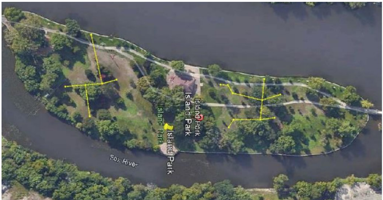
Island Park showing proposed drainage lines and catch basins
