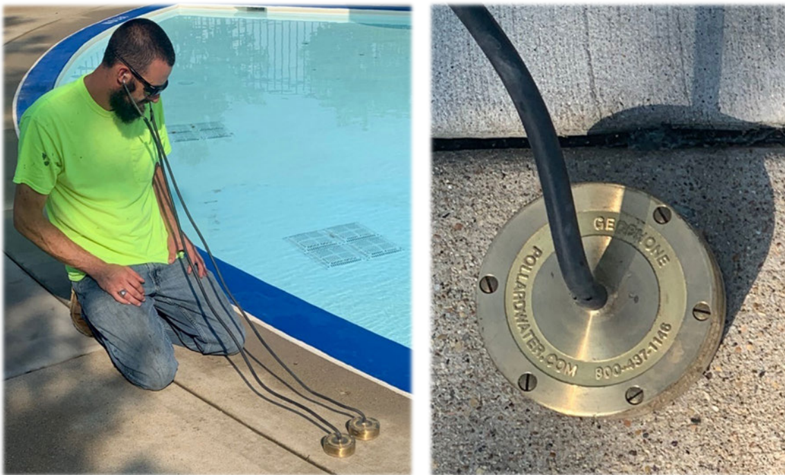
A technician uses a "Geophone" to listen for water leaks below ground
